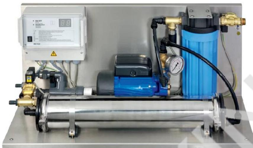
**Under sink or bench unit** for the desalination of softened drinking water (free chlorine not detectable), operating using reverse osmosis (RO). Drinking water can also be desalinated without pre-treatment. However, in this case the recovery rate is reduced. The decisive factor is the water analysis.
